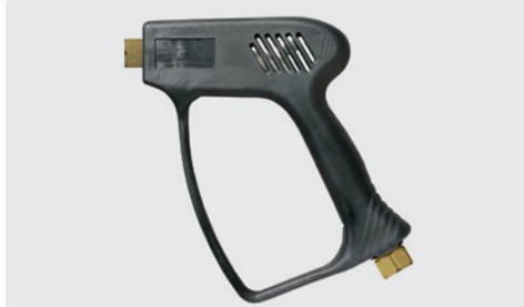
Professional gun without valve. Max. 275 bar / 45 l/min / 150 °C
